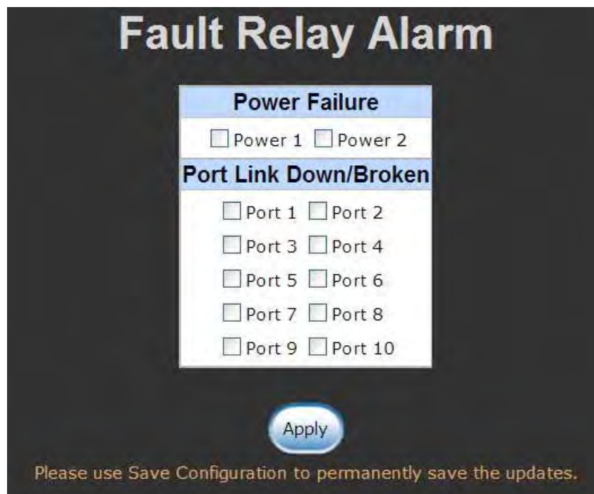
Fault Relay Alarm interface
