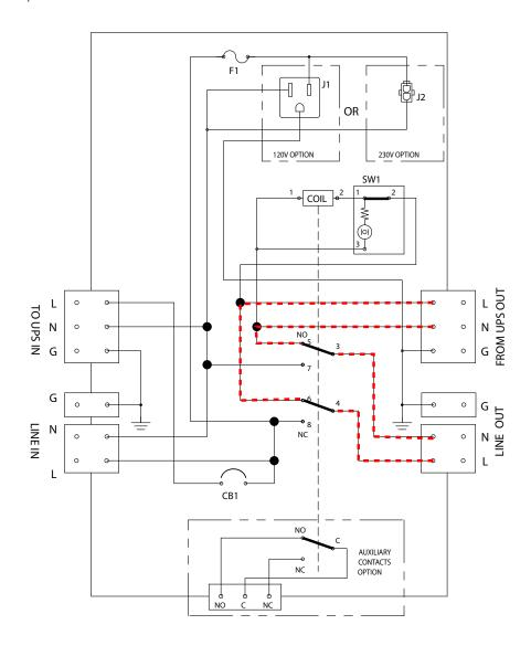
Figure 6.4 – UATS Operating in Inverter mode (SW1=Closed, CB1=Opened)
