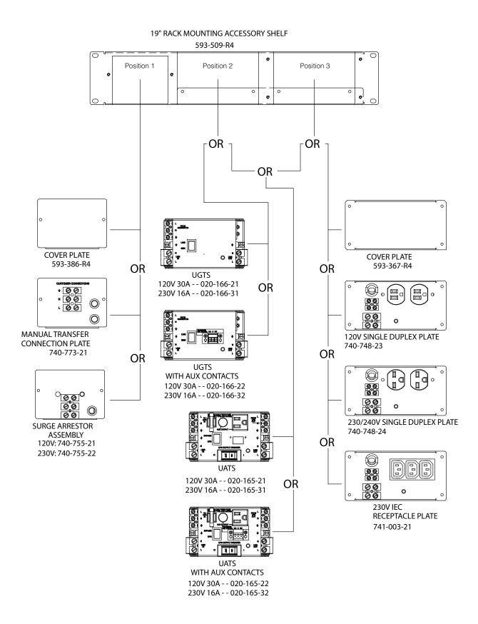
Figure 5.7 – Rack mounting Accessory Shelf - possible combinations
