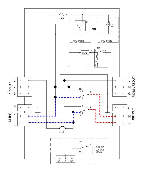
Figure 6.2– UATS Operating in Bypass mode (SW1=Opened, CB1=Closed)
