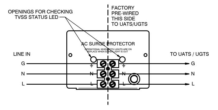
Figure 5.10 – Wiring the Surge Arrestor Plate
