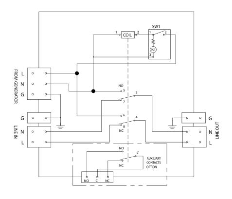
Figure 6.5 – UGTS Schematic
