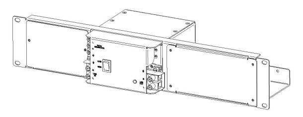
Figure 5.3 – UGTS in 19" Rack Mount Accessory Shelf
