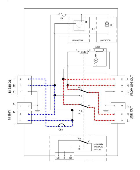
Figure 6.1– UATS Operating in UPS mode (SW1=Closed, CB1=Closed)
