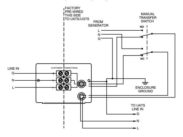
Figure 5.11 - Wiring the Manual Transfer Plate
