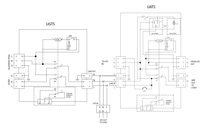
Figure 6.6 – UGTS wiring diagram with OR without UATS
