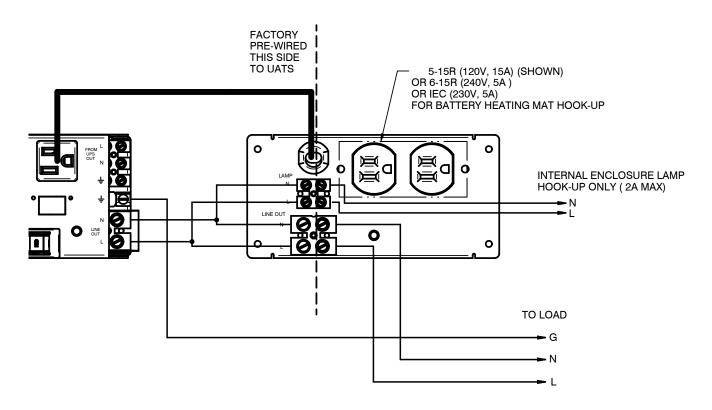
Figure 5.12 – Wiring the Receptacle Plates
