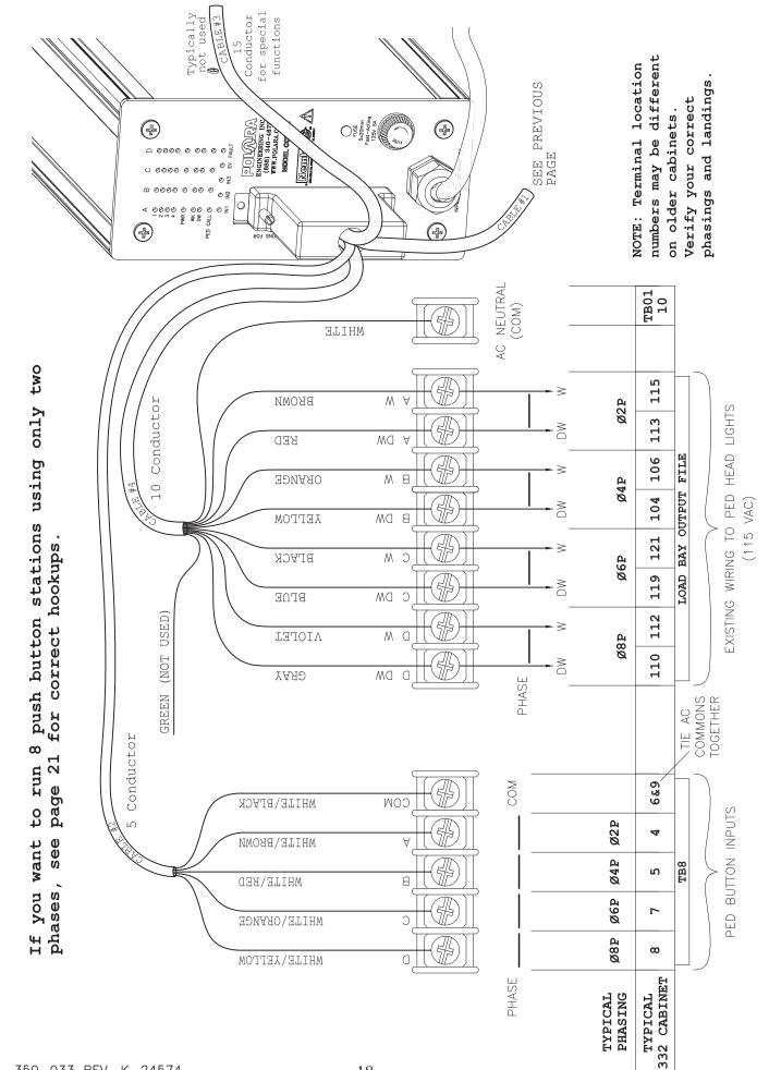
CCU2EN and Interconnect Board Cabinet Wiring (Cont.)
