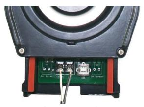
Wires connected to terminal block.
