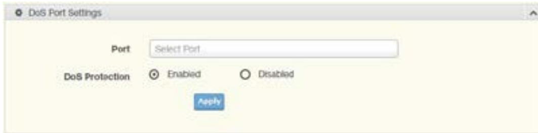
Figure 3.57 Security > DoS Prevention > DoS Port Settings
