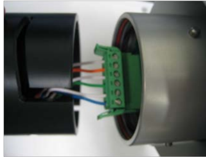
Wired Connector Plug in Place
