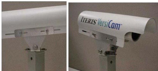
Camera Installed on Pedestal Bracket
