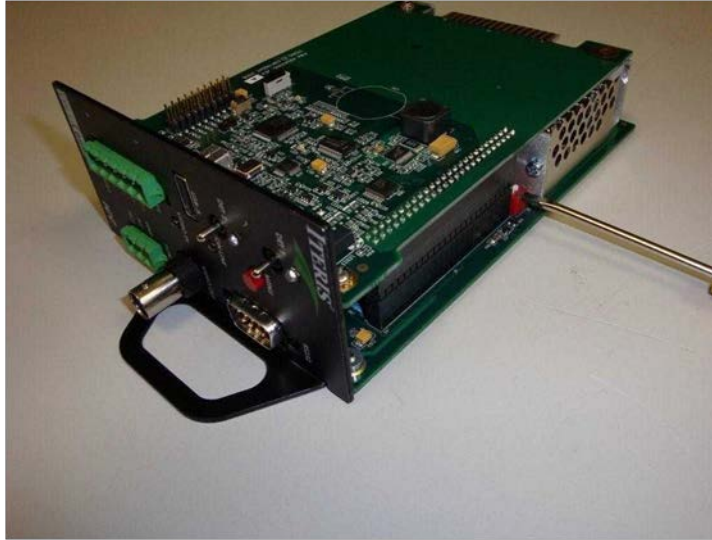
Screwdriver Pointing to the DIP Switches On VersiCam Module
