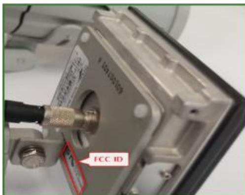
FCC ID Location on Back of Radar
