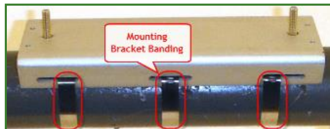
Banding Mounting Bracket to Arm
