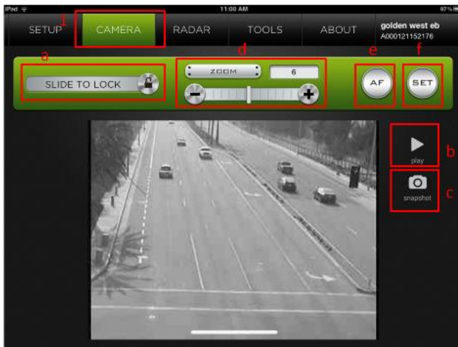
Camera Zoom & Focus Adjustments
