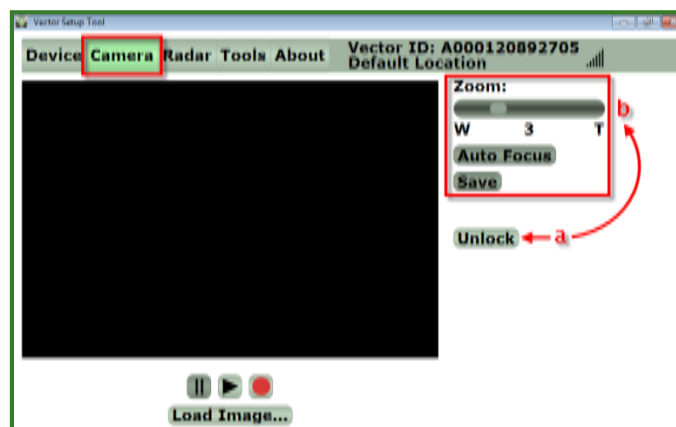
Adjusting Camera Zoom & Focus
