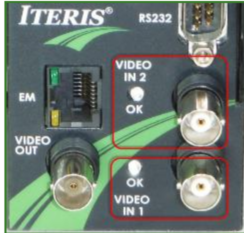
Attaching Coax to Processor Video In
