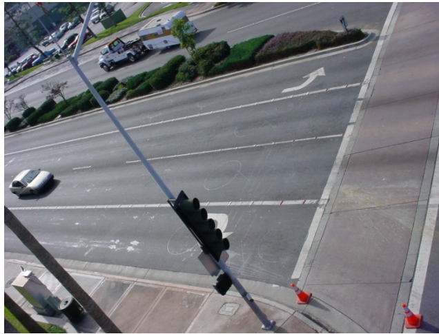
Very Poor Mounting - Side Shoot, Camera Not Centered
