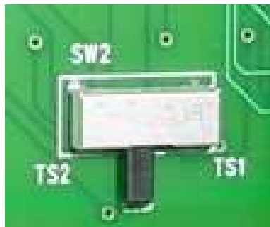
Toggle Switch SW2 for Rack Slot 4 Shown in the TS 2 Position
