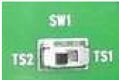
Toggle Switch SW1 for the BIU Slot Shown in the Default TS 2 Position
