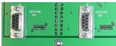
DB-9 Contact Closure Outputs for Processor Slots 1 - 3
