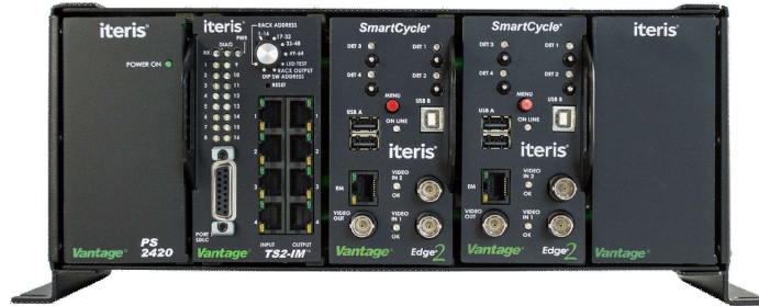
TS 2 VRack with Power Supply and Two Edge2 Processors
