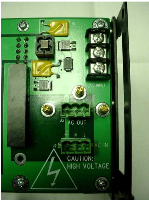
AC Protective Cover Removed
