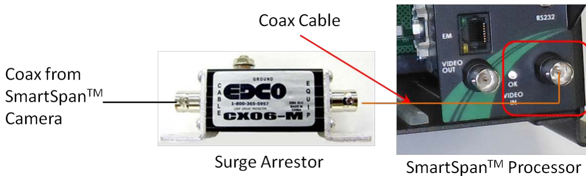
Attaching Coax to Processor Video In
