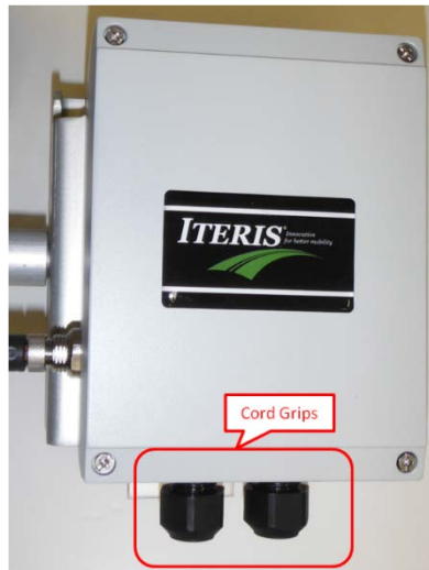
Tightening Cord Grips
