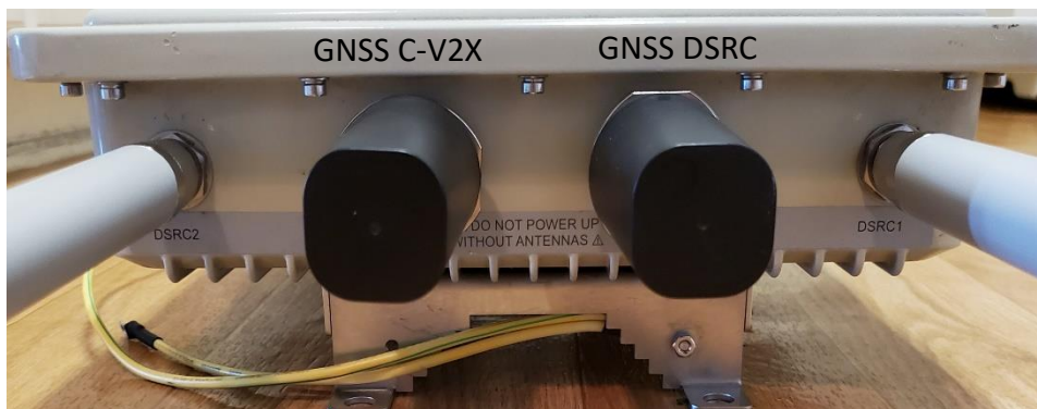
Figure 4: ESCoS Dual Mode DSRC/C-V2X RSU top view
