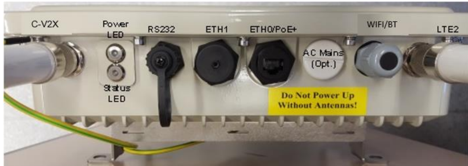
Figure 3: ESCoS Dual Mode DSRC/C-V2X RSU top view
