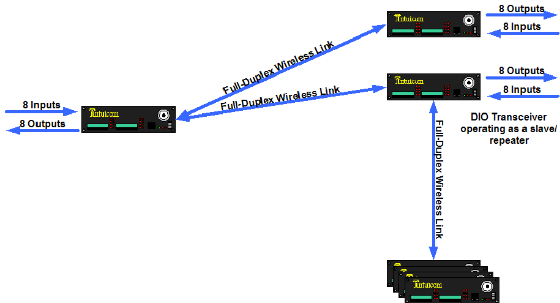
Figure 2-3: Point to Multipoint with Repeater
