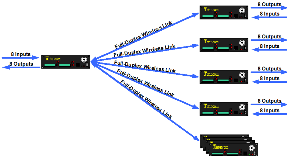
Figure 2-2: Point to Multipoint Network Architecture
